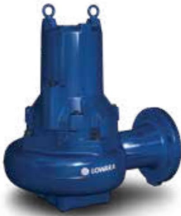
1315 Non-clog Maximum flow 54 l/s Maximum pressure 30 m Motor Rating 1,8 - 4,4 kW Outlet 80 - 100 mm Weight 80 - 84 kg
