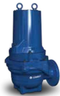
1320 Vortex Maximum flow 54 l/s Maximum pressure 29 m Motor Rating 3,5 - 7,5 kW Outlet 80 - 100 mm Weight 125 - 134 kg
